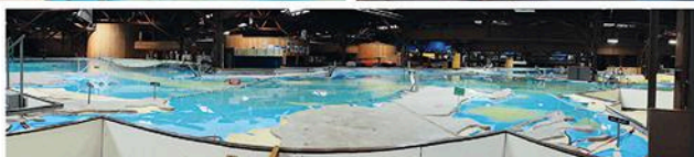
The Bay-Delta Model, built by the U.S. Army Corps of Engineers, is a working hydraulic model of the San Francisco Bay and Sacramento-San Joaquin River Delta System.
